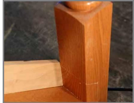
3. Mark the angles of the top and bottom post to both ends of the Mould with a pencil.
