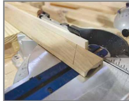
5. Make sure the Inserts are in the Handrail. Lay the Mould back on the side of the Handrail. The Mould should fit along the Handrail grooves perfectly. Since the Mould is cut, it is shorter than the Handrail.
