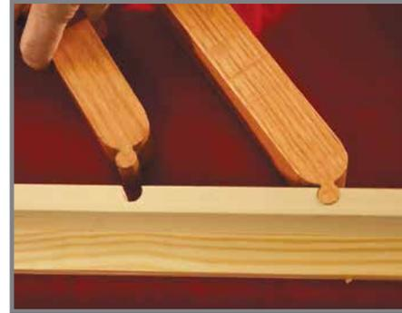
5. Once all the Balusters are in the Inserts, keep the entire assembled section at an angle and on top of the Support Strip, and then press the Precut Fillets between each Baluster except over the predrilled holes at the ends of the Inserts and also at the center of the Top Insert.
